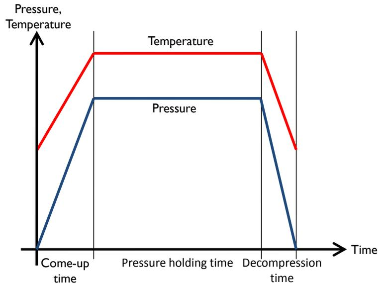
**Figure 1.** Pressure and temperature profile during a typical HPP treatment applied to food.
