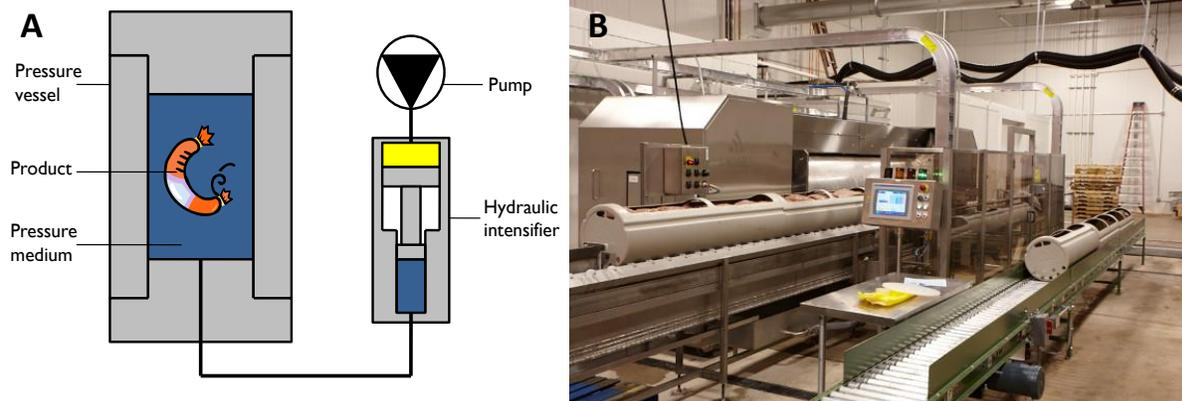
**Figure 2.** Schematic of an HPP system (A) and actual photograph of a batch HPP system owned and operated by American Pasteurization Company (B).
